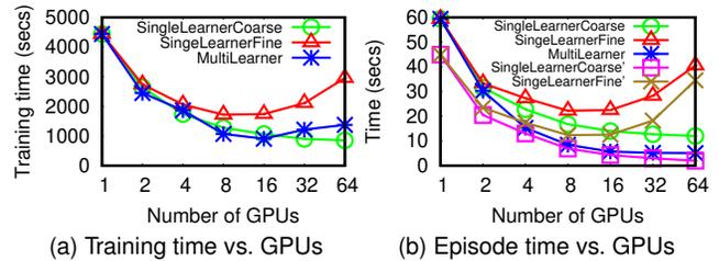
Fig. 9: Impact of GPU count on distribution policies
